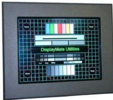
Model AS170P4HB2 is a true Daylight Readable (even in direct sunlight) high-quality industrial LCD system offering NEMA 4 (IP65) level protection at the front bezel. The product boasts a 17" display size with 1280 x 1024 pixels, 1200 nits brightness (long-life LED backlight) and 700:1 contrast ratio. This industrial grade Sunlight Readable NEMA 4 IP65 LCD TFT monitor is designed for use throughout a wide range of harsh outdoor applications.
