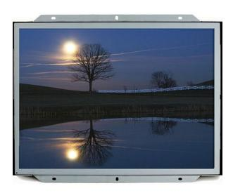
Model SRD-CM-104 is a rugged Sunlight Readable High Brightness Open-Frame systems with ultra-wide operational temperature capabilities. The product boasts a 10.4" display size with 1024 x 768 pixels, 1300 nits brightness (long-life LED backlight) and 700:1 contrast ratio.
